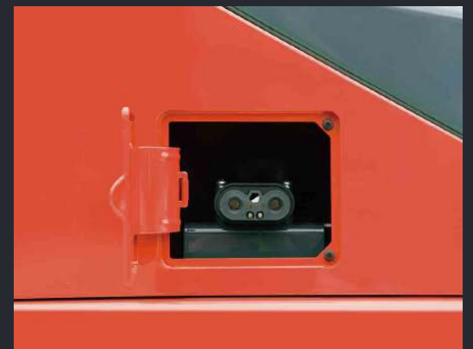
Multiple charging methods, with a standard REMA interface and an optional Chinese national standard charging interface.
